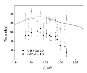
FIG. 7. Phase of the experimental signal for the LO modes as a function of  $E_c$ . The solid (dashed) line is the SRS phase calculation for the CdSe-like (CdTe-like) LO.
