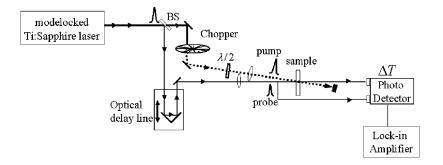
FIG. 2. Schematics of a pump-probe experiment. BS: beam splitter,  $\lambda/2$ : half waveplate. The pump pulse is modulated with a mechanical chopper. The probe pulse goes through the optical delay line. Pump and probe beam polarizations are perpendicular to each other, to reduce the pump scattering into the detector. The total transmission of the sample is measured using a balanced photodiode detector.
