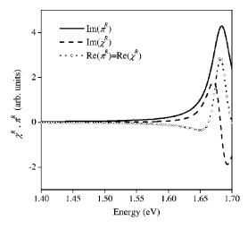
FIG. 9. Real and imaginary parts of the stimulated  $\pi^R$  and spontaneous  $\chi^R$  Raman susceptibility tensors. The calculation was performed using the dielectric function of a semiconductor QD of radius 39 Å (average radius of the sample). The tensors differ in their imaginary parts. Note that, at the resonance frequency,  $\text{Im}(\pi^R)$  is maximum whereas  $\text{Im}(\chi^R)$  is zero.
