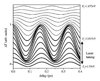
FIG. 10. Calculated total differential transmission  $\Delta T$  for a single mode as a function of the probe delay for different central laser energies,  $E_c$ . The calculation takes into account the dot size dispersion. A single phonon frequency was considered for all the dot sizes. The arrow indicates the range of  $E_c$  covered by our experiments. A clear resonant behavior is observed.
