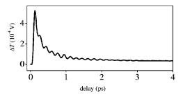
FIG. 3. Coherent phonon signal for CdTe $_{0.68}$ Se $_{0.32}$  QDs at room temperature. Typical differential transmission signal  $\Delta T$ , taken at laser central energy  $E_c$ =1.587 eV. The coherent phonon vibrations are superimposed on an exponential electronic background.
