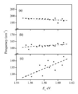
FIG. 8. Frequency of the LO phonons as a function of  $E_c$  (eV). (a) CdSe-like LO phonon, (b) CdTe-like LO phonon and (c) TO-LO mode. Full circles are experimental values and dashed lines are guides to the eye.
