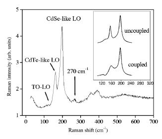
FIG. 11. Spontaneous Raman spectrum recorded at 514 nm. A weak indication of the TO-LO is seen at ~140 cm<sup>-1</sup> and the second order of this mode is resolved at 270 cm<sup>-1</sup>. The CdTe-like LO lineshape shows an asymmetry due to coupling with the TO-LO mode. The upper trace of the inset shows the calculated Raman lineshape for three independent oscillators. The lower trace of the inset shows an example of the Raman lineshape for two coupled oscillators and one independent mode.
