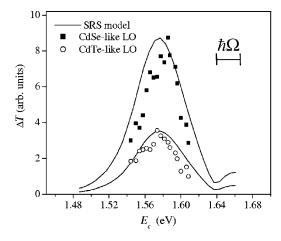
FIG. 6. Amplitude of the LO coherent phonons as a function of  $E_c$ . The full squares and the open circles are the amplitudes for the LO optical modes gained from the LP fitting. Solid lines show the impulsive stimulated Raman scattering (SRS) calculation, shifted to lower energies by 20 meV. The CdSe-like LO phonon energy is indicated as  $\hbar\Omega\!\approx\!25$  meV.
