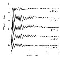
FIG. 5. Differential transmission  $\Delta T$  as a function of the probe delay for different laser central energies  $E_c$ . The data was normalized to a common laser power. The curves are shifted vertically for clarity.
